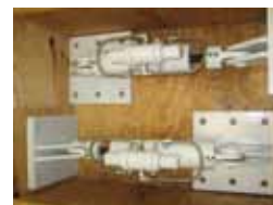
Transpec hydraulic dampers without seal
